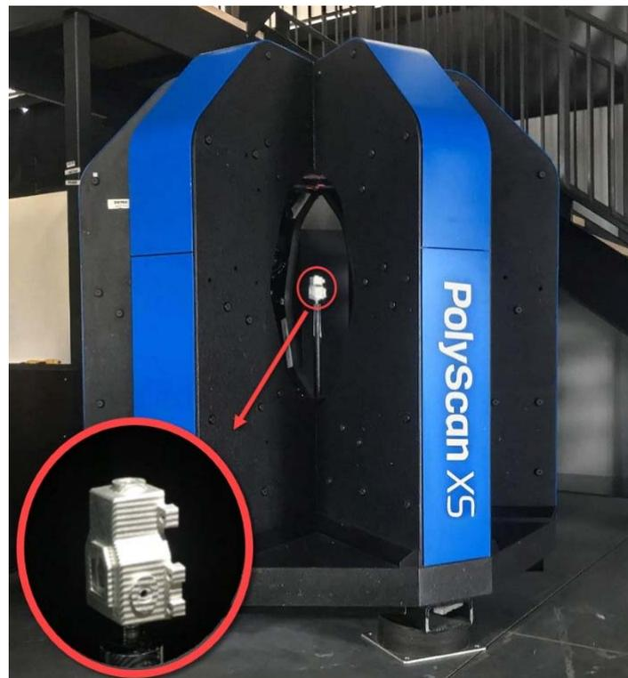
Figure 2: First 3D-printed sample being scanned in the PolyScan XS
