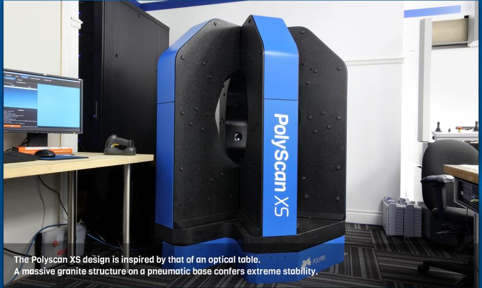
The Polyscan XS design is inspired by that of an optical table. A massive granite structure on a pneumatic base confers extreme stability.
